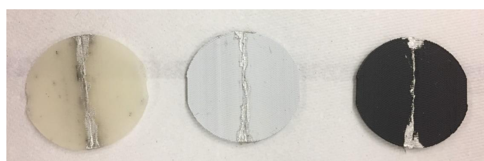
Oriented circular samples for thermal conductivity testing for pure PLA (left), 90/10 PLA/BN (middle), and 90/10 PLA/GNP (right)
